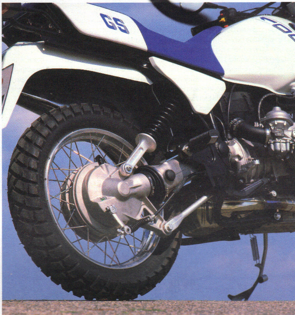
Rear floating was much improved by this clever arrangement; retaining the easy-removal wheel attachment and single-sided swinging arm; the Paralever
